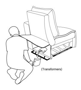
STEP 3: Connect the Transformers (A) to the Power cord
